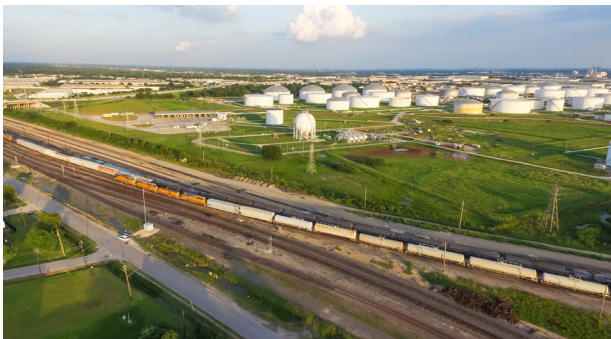
Aerial view of tank farm for bulk petroleum and gasoline storage next to rail line in Northeast Houston (Photo: Shutterstock/ Trong Nguyen)
